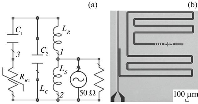
**Fig. 1.** (a) Equivalent circuit of an RFTES with a frequency selection circuit. (1, 2) The input and output ports of the chip and (3) the port for connecting the bridge. (b) RFTES detector in a resonator matched according to the 50  $\Omega$  standard. Gray color corresponds to metal; black color, to the substrate.
