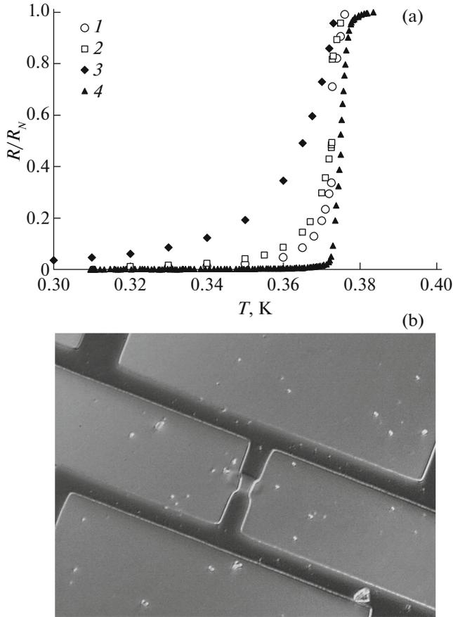
**Fig. 2.** (a) The real (active) part of the normalized high-frequency impedance of a hafnium bridge at frequencies of (1) 1, (2) 1.5, and (3) 5 GHz in comparison with (4) direct-current measured ratio  $R/R_N(T)$ . (b) Photograph of a hafnium microbridge embedded in a quarterwave resonator.
