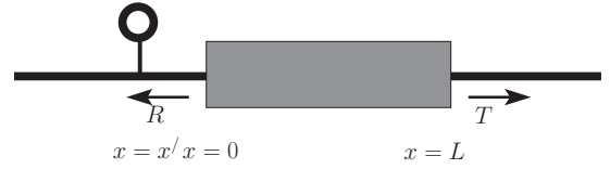
FIG. 6. Sketch for the Green's function calculation. The “black box” is characterized by transmission and reflection coefficients. The source (Dirac delta) is represented by the ring attached to the line.
