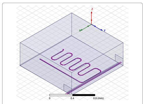
Figure 3 CPW resonator and feedline model used for 3D numerical simulation. The isolated sections of the resonator waveguide are bent into a meander for compactness. Only the length of the straight coupler section is included in  $I_c$ . The lengths of the arcs are included into the lengths of the shorted and open ends of the resonator  $I_s$  and  $I_o$ .
