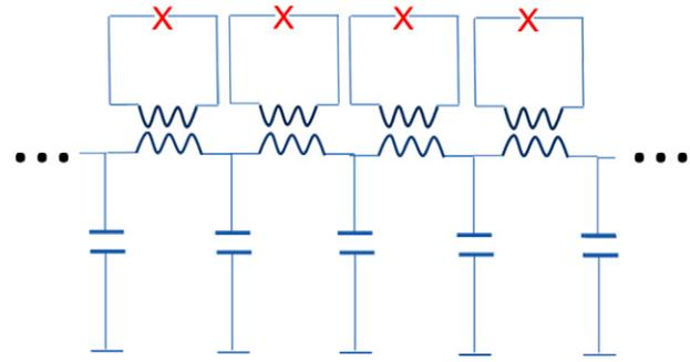
**Figure 1.** The schematic of an array of RF SQUIDs incorporated in a transmission line.
