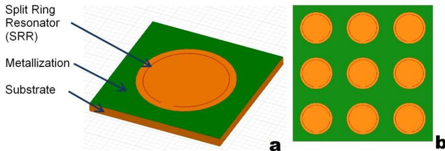
Fig. 1. (a) General view of the FSS unit cell. Unit cell consists of a silicon substrate (orange) and of metallization with a round aperture (green). The NbN split ring resonator is placed into the aperture (red). (b) A top view of the FSS with 3x3 unit cells.
