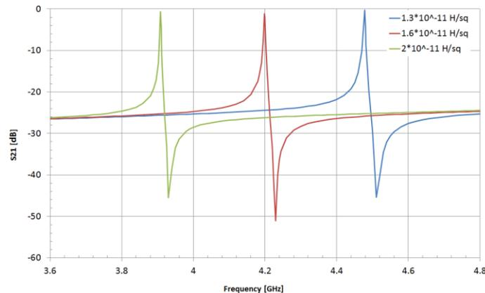
Fig. 2. Transmission (S21) through the designed FSS simulated with HFSS software for the normal incidence of a flat wave. The transmission is calculated for the kinetic inductance value at the temperature far below the critical temperature  $T_c$  ( $L=13$  pH/sq (blue line)) and for the temperature near  $T_c$  ( $L=20$  pH/sq (green line)). Predicted resonance frequency shift is about 15%, from 4.5 GHz to 3.9 GHz. Note a 100 % transmission at the resonance frequency of the tunable FSS.
