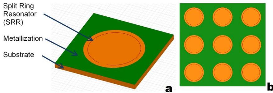
Fig. 1. (a) General view of the FSS unit cell. Unit cell consists of a silicon substrate (orange) and of metallization with a round aperture (green). The NbN split ring resonator is placed into the aperture (red). (b) A top view of the FSS with 3x3 unit cells.
