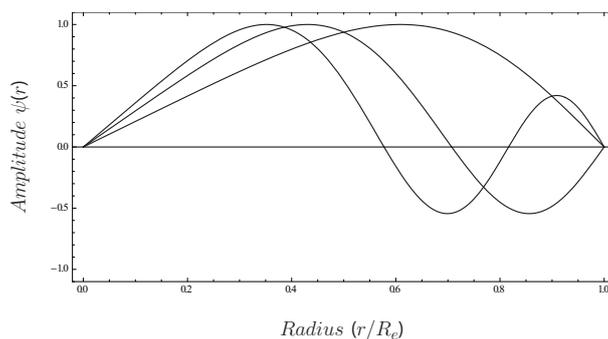
Fig. 2: The current distribution across the spiral turns for first three resonance modes.  $\psi(r)$  normalized to maximum value equal to one.
