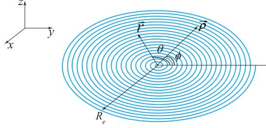
Fig. 1: A sketch of a spiral resonator with many turns. The polar coordinates  $\rho, \varphi$  (the coordinates of the point on spiral), and  $r, \theta$  (the coordinates of the observation point in the plane of the spiral) are shown.  $R_e$  is the external radius of spiral.
